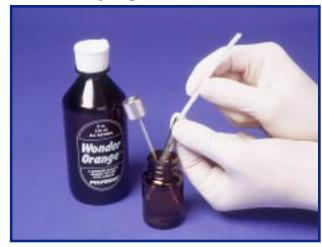
Immediately after use, separate the screw plunger from the barrel by turning the plunger counterclockwise. Use Wonder Orange Cleaning Solution to clean the screw plunger and barrel. A pipe cleaner can be used to help clean the inside of the barrel. When the Pressure Syringe is clean, the screw plunger should spin freely in the barrel.
